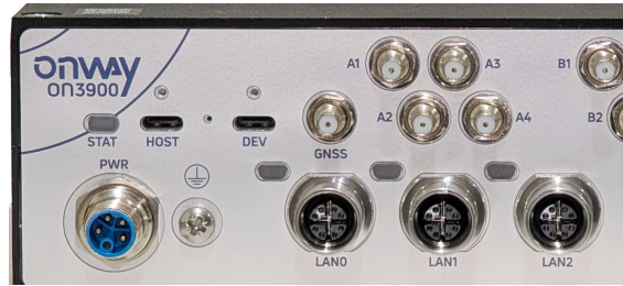
ON3900 Router Front View. The STAT LED is on the upper lefthand side and the Ethernet LEDs are above each port on the left.
